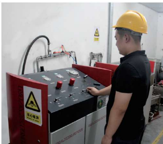
超高压工业软管总成试压工序 Pressure Test for Industrial Hose Assemblies
